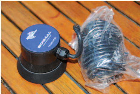
The transducer, straight out of the box. The tightly coiled cable aids installation in tight places
