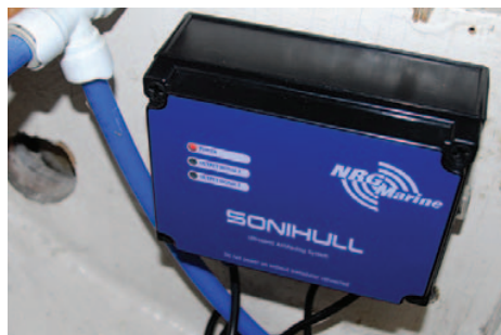
You can mount the control box anywhere within reach of the transducer cables
