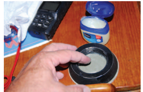
I smeared Vaseline into the threads and applied a thin layer to the mating surface to get rid of air bubbles that might inhibit transmission
