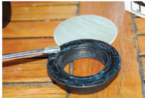
I applied epoxy resin to the mounting ring then clamped it to the G10 disk overnight
