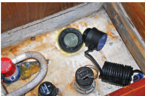
I epoxied the mounting ring on its G10 disk to the hull, first sanding the area down to provide a key for the thickened adhesive
